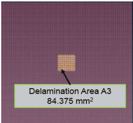
Fig. 3. Top view of delamination incorporated.
