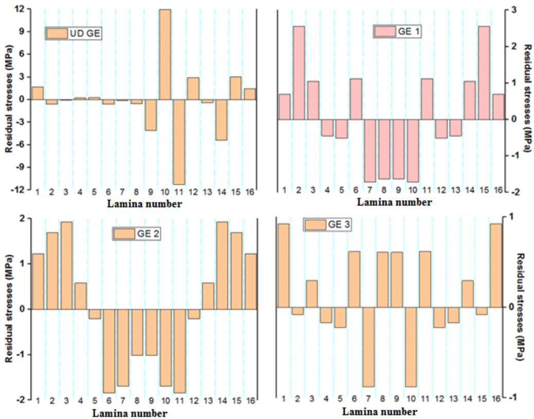
Fig. 7. Longitudinal residual stress in each lamina of GE laminates.
