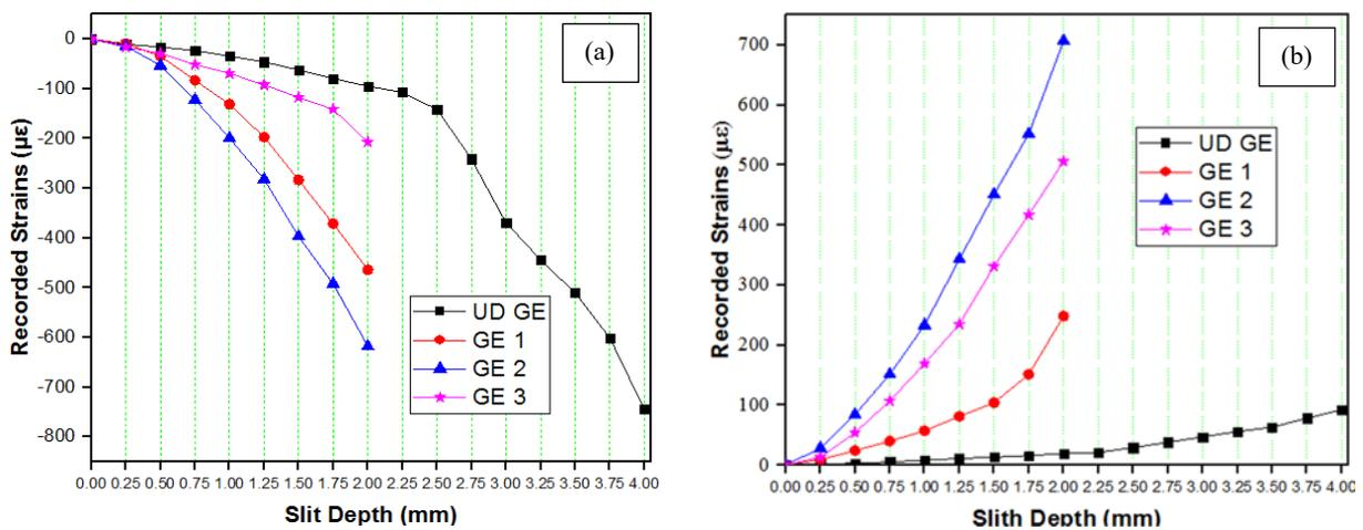
**Fig. 6.** (a) Strains recorded along with the laminate depth during slitting of all GE longitudinal specimens. (b) Strains recorded along with the laminate depth during slitting of all GE transverse specimens.
