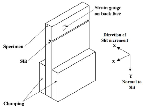
**Fig. 3.** Details of Slitting Specimen
