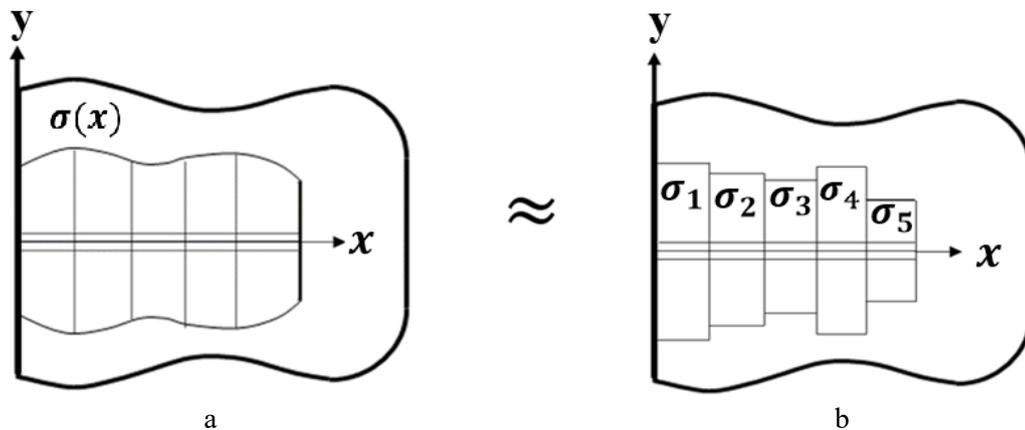
Fig. 4. (a) An unknown residual stress profile on slit faces; (b) A series of uniform strip loads are used to approximate the Unknown residual stress.
