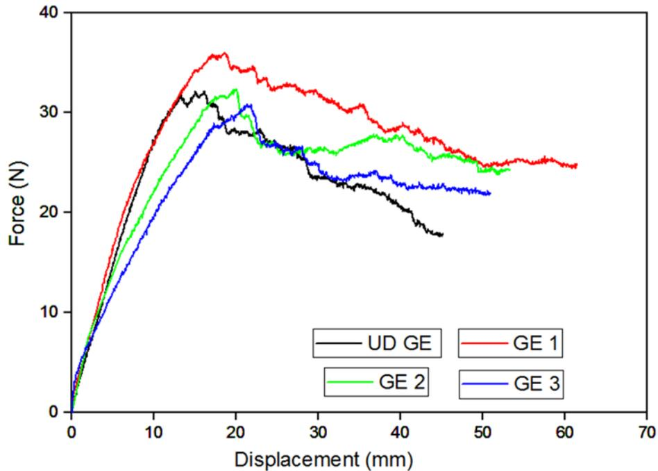
Fig. 9. Load-displacement plots of GE laminates
