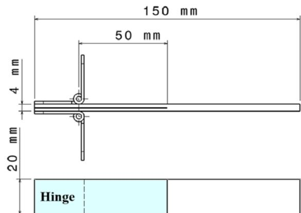
Fig. 2. Geometrical dimensions of DCB specimen
