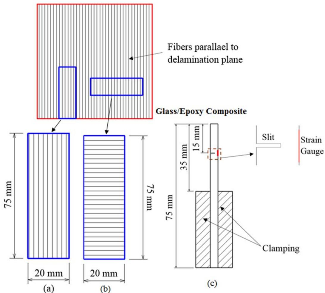
**Fig. 5.** (a) Slitting specimen used to determine longitudinal residual stresses in composite laminate (b) Slitting specimen used to determine transverse residual stresses in composite laminate (c) Slitting specimen with a bonded strain gauge.
