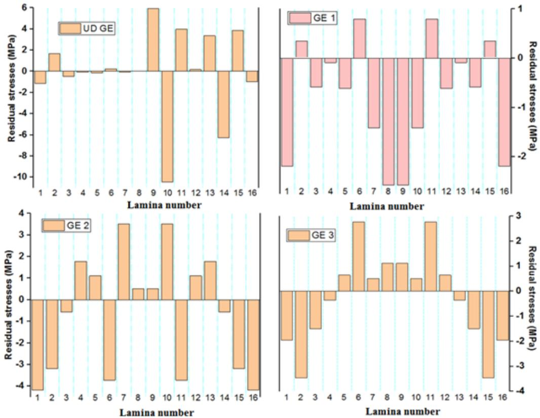
Fig. 8. Transverse residual stress in each ply of GE laminates.
