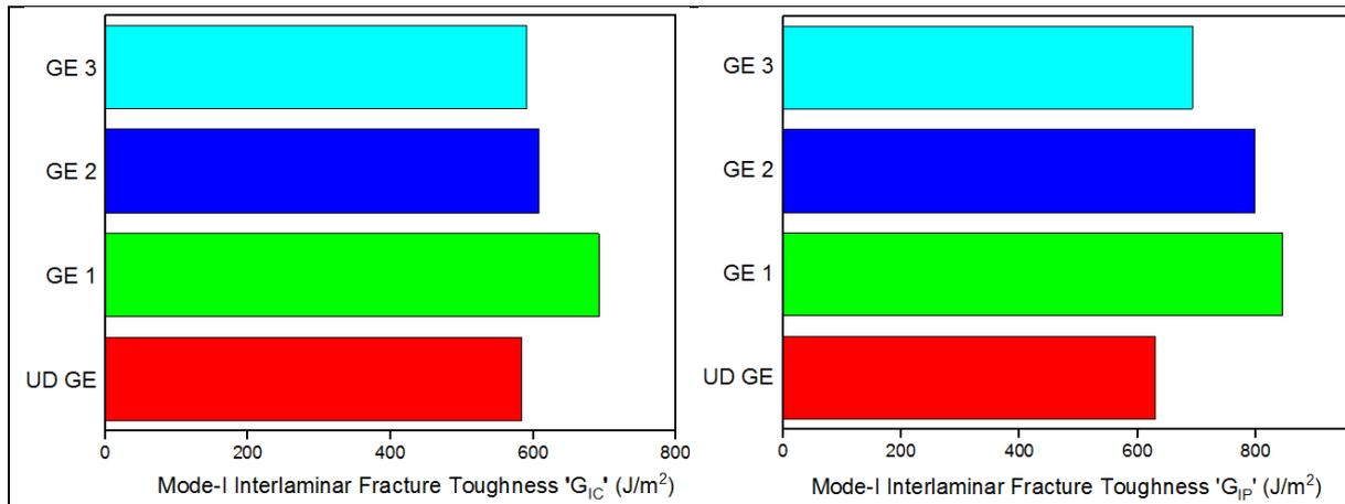
Fig. 10. Mode I interlaminar fracture toughness for initiation ' $G_{IC}$ ' (Left) and propagation ' $G_{IP}$ ' (Right) of GE laminates
