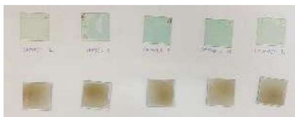
Fig. 2. Electrochemical deposition on ITO (before and after sulfurization– top-bottom)
