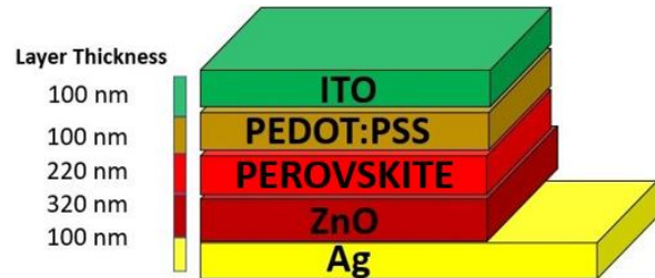
Fig. 16. Simulated Perovskite Solar cell with layer Thickness
