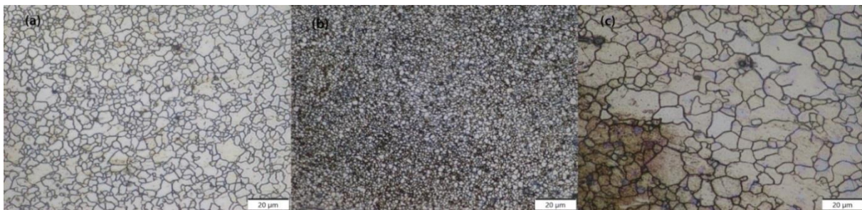
Fig. 18. Microstructures of Friction Stir Welded Joints: (a) 750 rpm, 10 mm/min, 15 mm, (b) 825 rpm, 15 mm/min, 18 mm, and (c) 900 rpm, 20 mm/min, 20 mm
