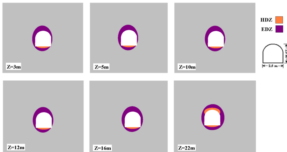
Figure 6. The EDZ and HDZ around different sections of a gallery, Gotvand dam
