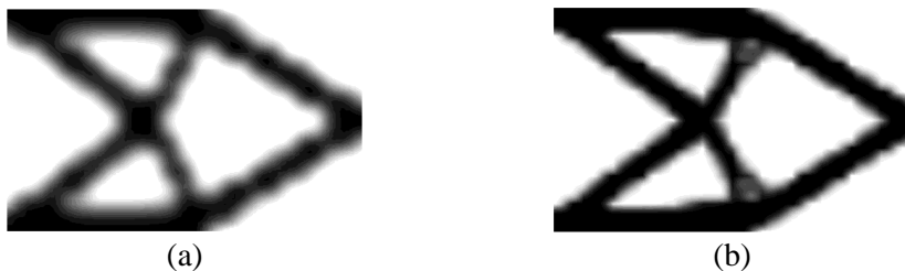
Figure 4. Optimum layout (a) by using 400, (b) 1617 control points [9]
