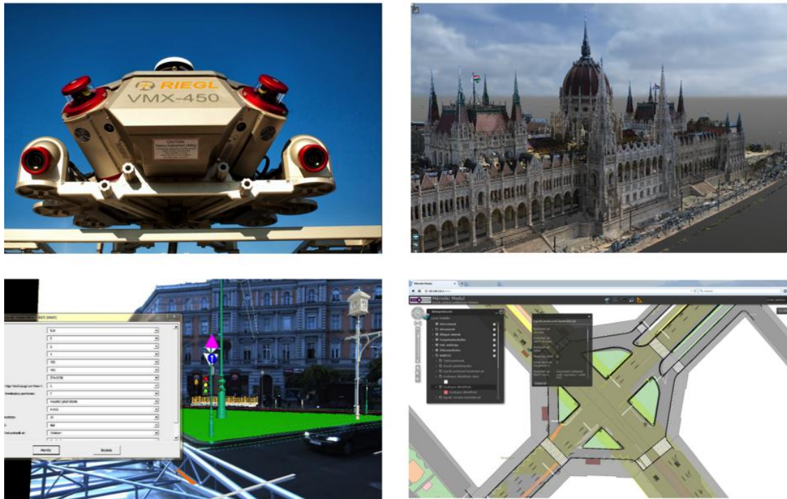
Figure 1. Main components of RODIS: VMX 450 scanner (top left), point cloud data (top right) 3D geodatabase (bottom left) 3D GIS portal (bottom right)
