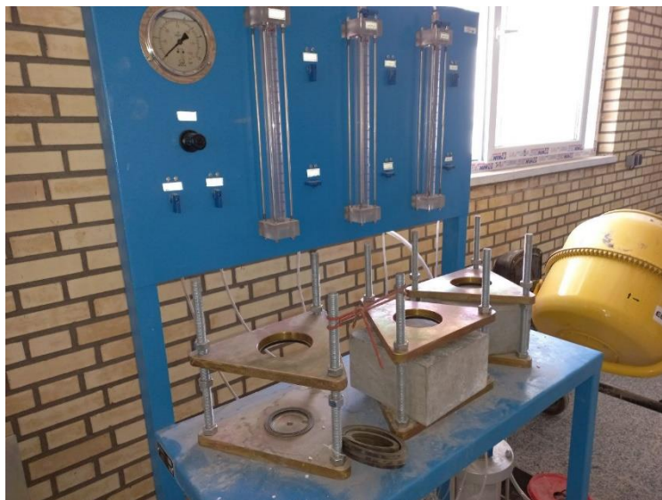
Figure 17 An image of the permeability test apparatus
