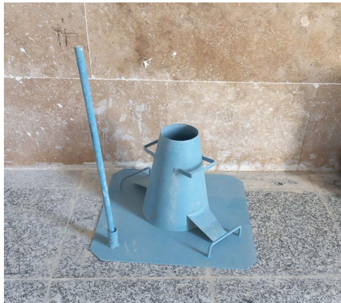
Figure 10. Slump test cone
