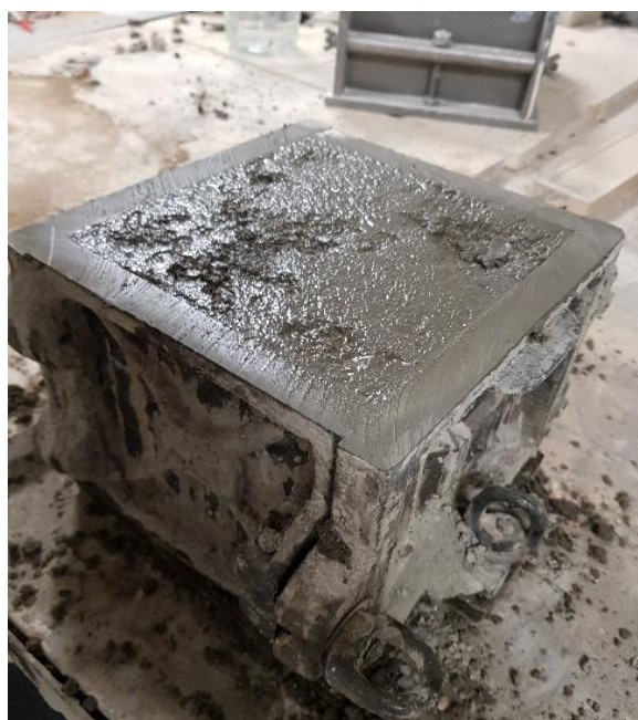
Figure 11. A 150 millimeter mold filled with concrete
