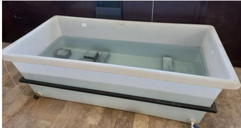
Figure 8. Concrete curing water bath
