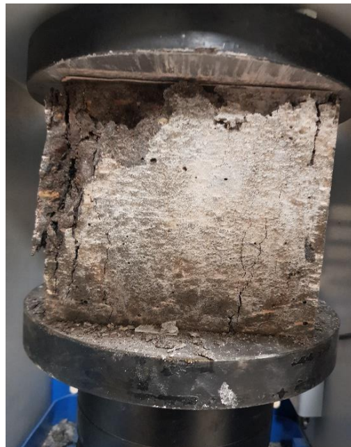
Figure 13. The failure pattern of the 90-day sample with 40% travertine sludge
